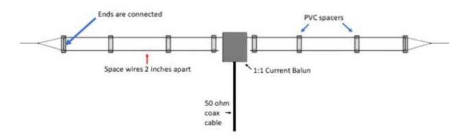
The overall length of this easy-to-build M0PZT version is 40 feet for the 40m band. It will also cover the 15m band. The feedpoint impedance for this configuration is about 35 ohms. Important: Keep the wires parallel. (Image/Mark, K8MSH)
