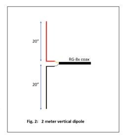
No matter which you choose, keep the coax run as short as possible to minimize power losses. Use a good quality coax like DXE RG-8x for short runs, RG-8 for longer runs.
