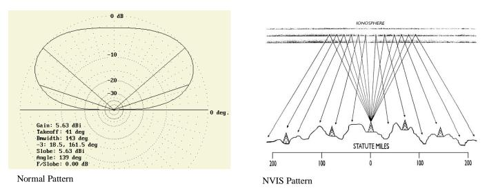
What do you do to get an NVIS pattern? The good news is it's not hard and can be as simple as taking an existing antenna and lowering it to only 10'-15' above ground. You can find details on the DX Engineering Website here:
