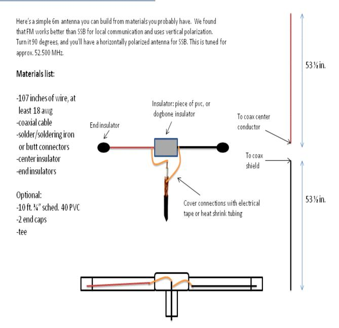
You can also enclose in PVC pipe. Instead, strip enough coax to push through the PVC tee connection. Connect antenna wires to the coax as shown above-- don't use the insulator. Cover with electrical tape or heat shrink tubing. Slide PVC tubing over wire and cap ends. To tower mount, slip an 18" piece of PVC in the end of the tee and run the coax through it. Connect to tower with U-bolts.
